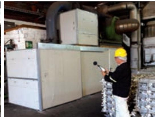
*Noise Measurement at aluminium factory*
